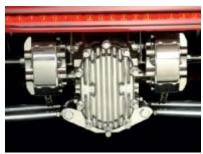
A custom rear license-plate bracket flips up and down at the touch of a switch to show off the polished IRS components.
